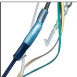
**Heat-Shrunk Sealed, Concealed Wiring**
