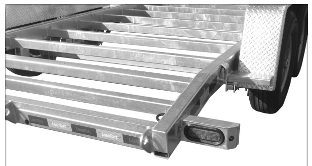
Typical galvanized trailer frame.
