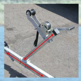
Fully adjustable winch and stand adjusts for length and height
