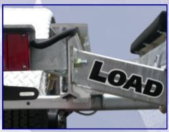
Custom extruded aluminum frame rails incorporate wire and fastener channels
