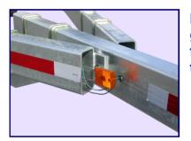
Massive 6" x 3" galvanized steel frame and tongue tubes
