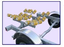
48 TPR rollers on special heavy-duty 8 roller trucks concentrated at the rear
